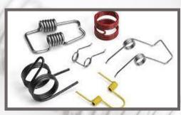
Double torsion spring comprised of two torsion spring coils which are connected in the centre to form a single spring. The two coils are wound from a single piece of wire in opposite directions, with one wound counter clockwise and the other clockwise.
